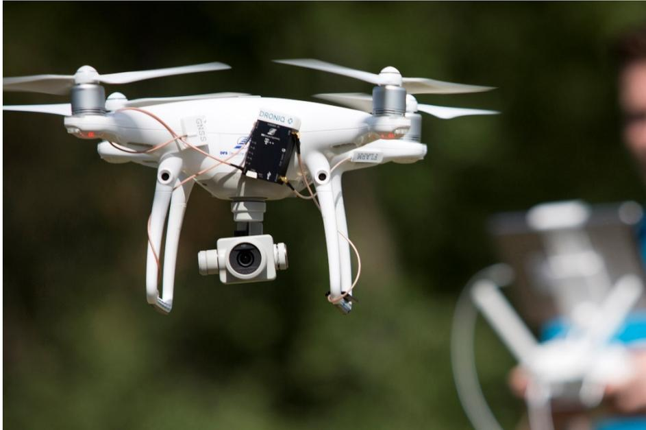
Picture 1: Drone with Hook-on-Device for the UTM system of DFS (© Deutsche Flugsicherung GmbH)
