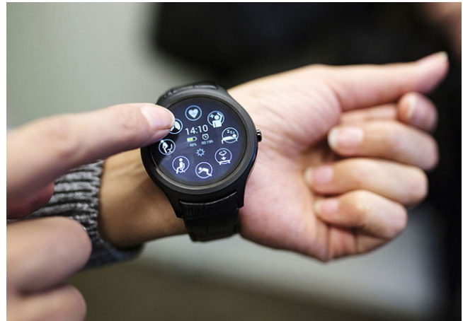
Figure 1. We present a Mobile Assisted Living Smartwatch-app, which runs on a No.1 D5+ Android watch. Implemented features include the detection of: Respiratory Parameters, Cardiac Parameters, an explicit Help Gesture, Fall Detection, Sleep Parameters, Posture Parameters, as well as Gait and Activity Parameters. These parameters are used to calculate a fall risk level for the elderly.
