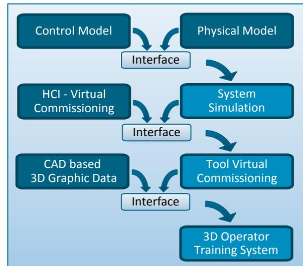
Figure 2: Three step concept for System Simulation, Virtual Commissioning and 3D Operator Training
