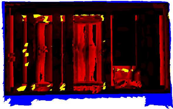
Figure 8: Color encoded differences of the reference 3D model and the reconstructed 3D model.
