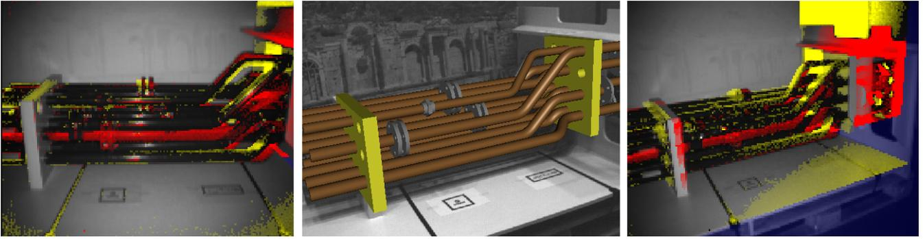
Figure 1: Center: One of the pipes is missing in the 3D model. Left and right: Color encoded visualization of the differences between the 3D model and the real scene.
