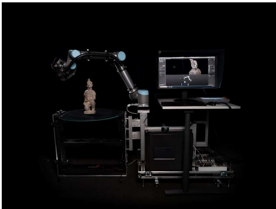
Photo: The autonomous, colour-faithful 3D scanning system CultArm3D GT10 by Fraunhofer IGD automatically and safely generates high-resolution 3D scans—perfect for use in museums. (© Fraunhofer IGD)
