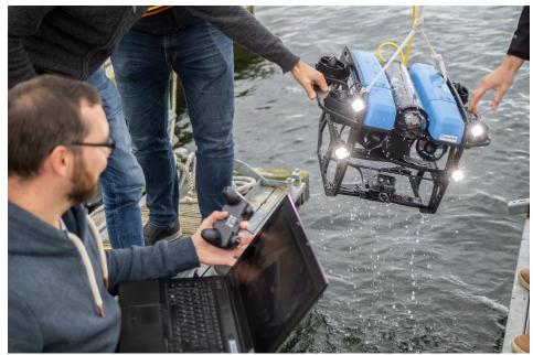
Image: The interdisciplinary Fraunhofer research team "Smart Ocean Technologies" in Rostock is working on underwater vehicles to analyze microplastics in the oceans. (Right of use: Fraunhofer IGD)
