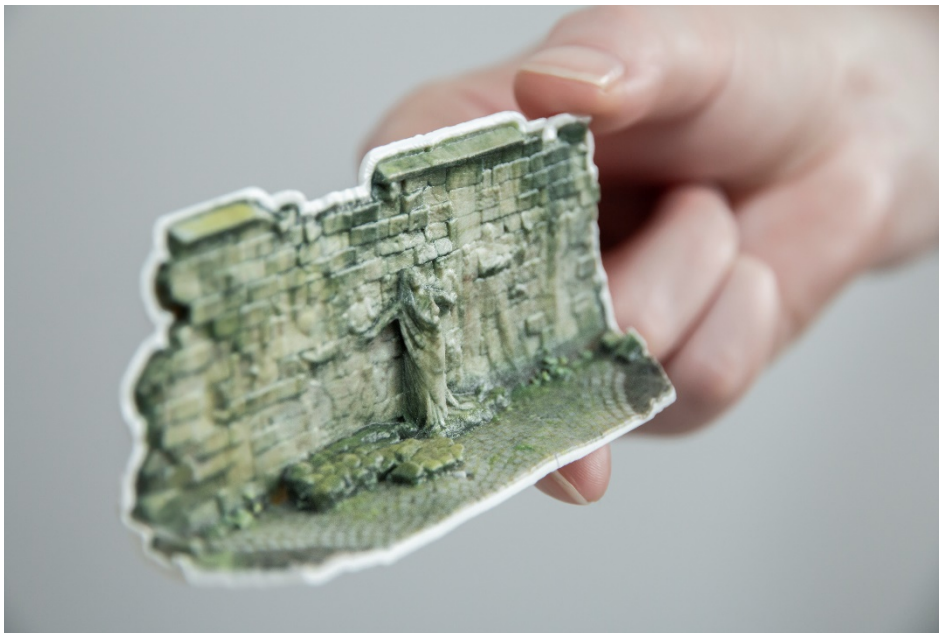
Image 1: On the Mimaki 3DUJ-553, Fraunhofer's 3D printer driver Cuttlefish helps produce highly precise prints in even the smallest of formats. (© Fraunhofer IGD)
