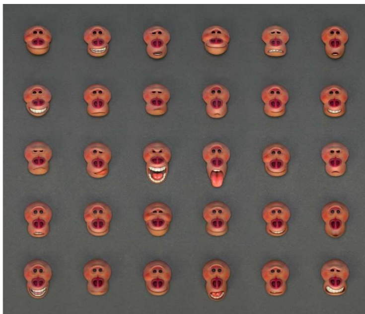
Image 2: Mr. Link's different faces and emotions were 3D-printed with the patented Cuttlefish technology of Fraunhofer IGD. (© LAIKA)
