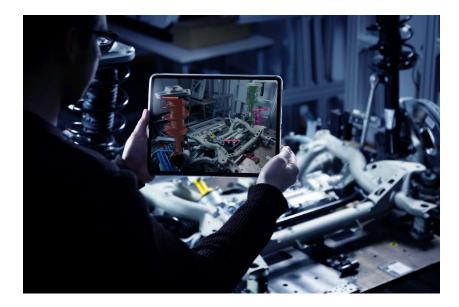
Image: Marquis from Fraunhofer is an all-round solution for reducing the time and effort involved in quality assurance. It provides visual inspection during the ongoing assembly process and can also map the associated documentation. (Source: Fraunhofer IGD)
