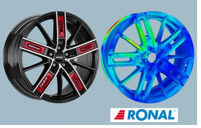
RISTRA accelerates the simulation of a rim designed by RONAL GROUP by a factor of 93.
