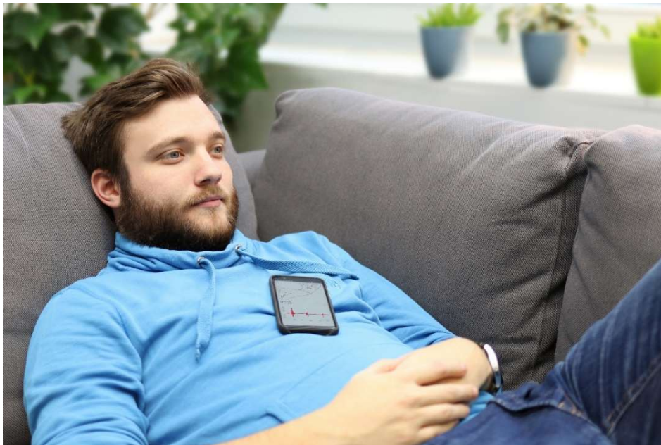
Image Caption: Fraunhofer IGD's Guardio® app records heart movements and translates them into a multi-channel ECG. (© Fraunhofer IGD)
